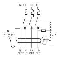
Will operate and is suitable for 4 wire motor circuits without the load neutral
