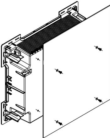
The section that extends outside the frame of the board is to protect the incoming mains cables. The plate can be reoriented to suit either direction.
