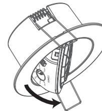
The Time1 and Lux setting are on one side, the Time2 and Sensitivity on the other. Note: TIME2 only needs to be adjusted if the Output #2 is connected to a load
