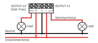
Sensor Controlling One 240Vac Load and a separate Low/Alternative **Voltage Load**
