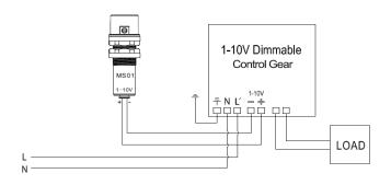
Connect the red wire(+) and black(-)of Sensor to the "+,-" of the dimmable cable of driver. Checking whether the wiring connection is right.
