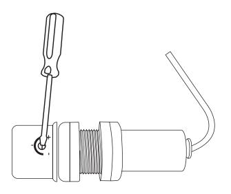
Turn the knob from "-" to "+", the lux value will be changed from 10lux to 800lux. Adjust the knob slowly and use the lux meter to detect the environment lux at the same time, then you can set the lux you want in the room.
