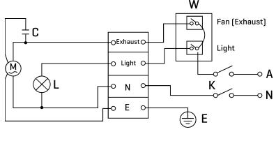
M: Motor C: Capacitor W: Wall switch(s) K: All-pole disconnection switch L: LED Driver & Light
